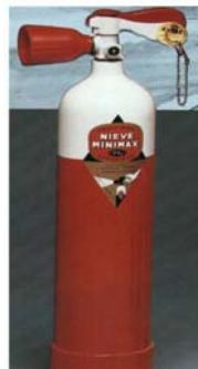
Used for type A fires (solids, such as paper, wood, etc.), type B (flammable liquids) and type C (gases such as propane, butane, etc.). It can also put out fires where there is an electrical installation, but powder can spoil the machines nearby.
